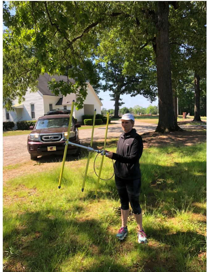
Mary Catherine Domaleski (KI4HHI) takes a reading northeast of Carrollton, using our tape measure Yagi attached to a Kenwood TH-D74. We stayed in contact with our team captain AI4RT using 146.535 MHz simplex to share bearings.
